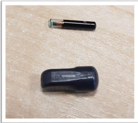
**A PIT tag (top) compared to a 5mm acoustic tag (bottom)**
