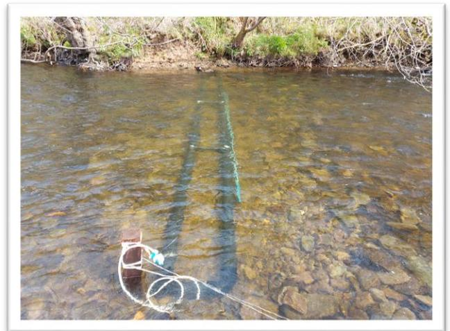
**A PIT antenna attached to the streambed in the lower Gala Water**
